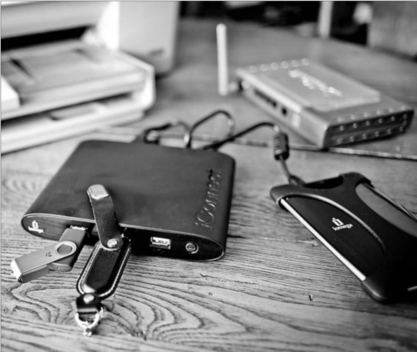
Central control: an iConnect linked to two memory sticks and a hard drive via the USB ports, and wirelessly to a router Pascal Perich Central control: an iConnect linked to two memory sticks and a hard drive via the USB ports, and wirelessly to a router
